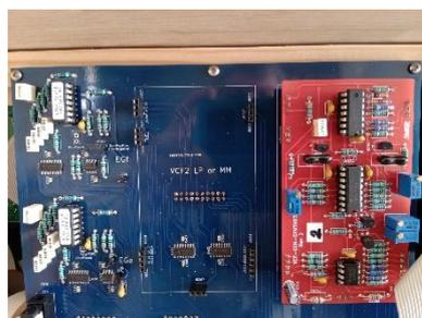
To replace another filter, align the connectors, if possible starting with the connector at the bottom of the card, then align all the contact points and push in the circuit, the cards must be aligned with the underlying silk-screen printing, then close the rear panel if necessary.
