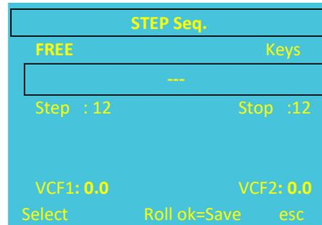
This is how the Sequencer Step screen looks before recording and then during recording. The note is displayed while playing the keyboard, then the next step is waiting.
